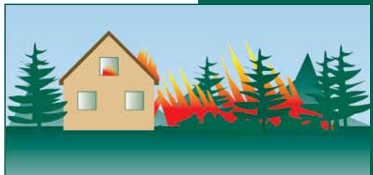
Figure 2-5: Fire directly impinging on a house
