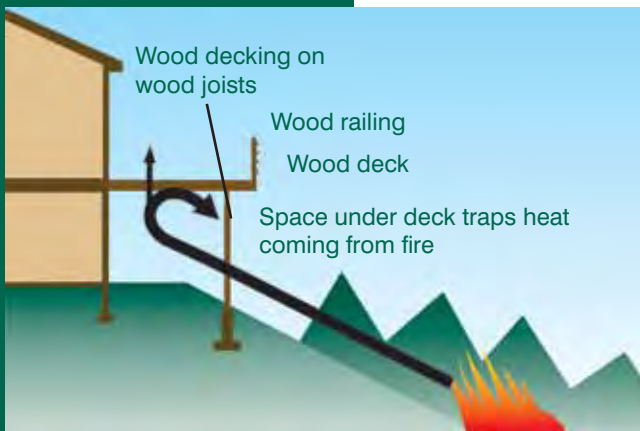
Figure 4-10: Conventional deck in a fire
