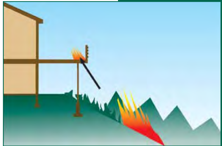
Figure 4-12: Conventional decks can easily ignite during a wildfire
