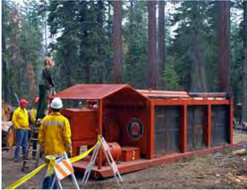
Model S-220 Air Curtain Destructor
