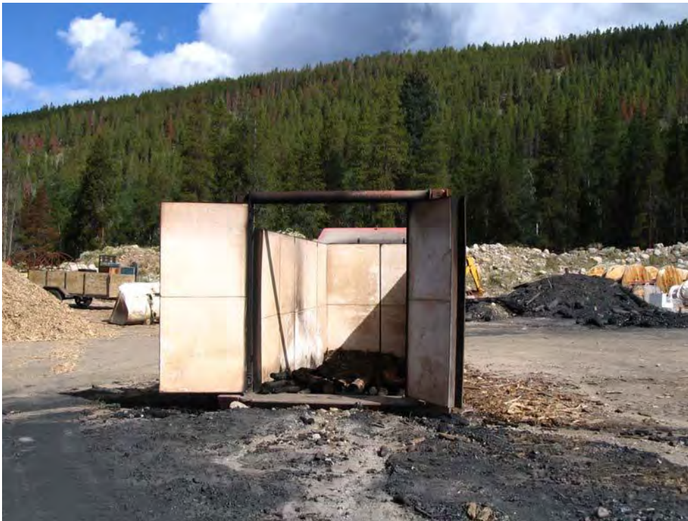
Model S-220 Air Curtain Destructor
