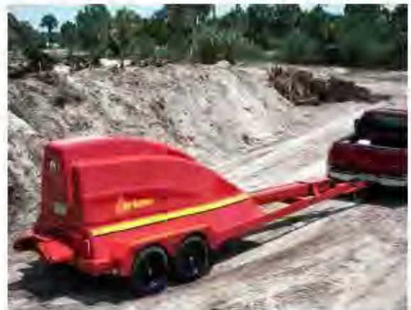
Figure 5—Trailer mounted trench burner system.
