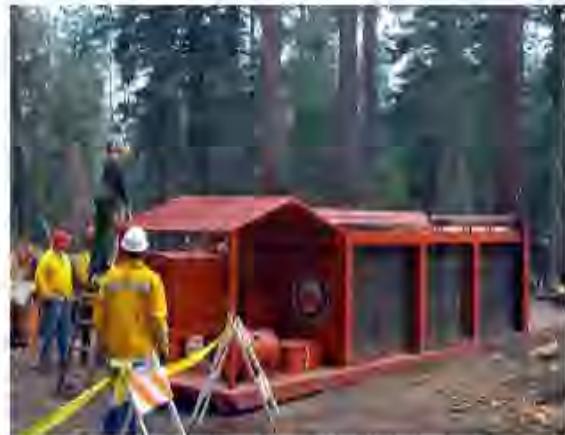
Figure 3—Skid mounted ACD in full operation (no visible smoke).
