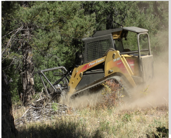
Machine mastication with skid steer
