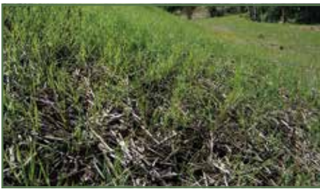
WoodStraw® is an erosion-control material made up of interlocking wood strands. Photo: Trent Jones
