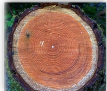
Figure 1. Cross section of a Douglas fir. The light colored outer ring of wood is the sapwood. The dark wood in the center is the heartwood.
