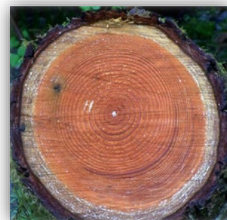
Figure 1. Cross section of Douglas fir. Light colored outer rings are sapwood. The dark wood in center is the heartwood.
