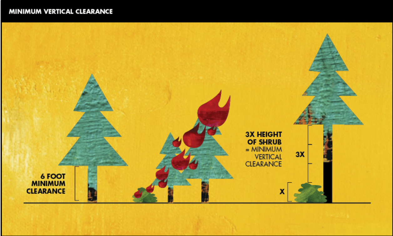
Figure D.3. Recommended minimal vertical clearance.
