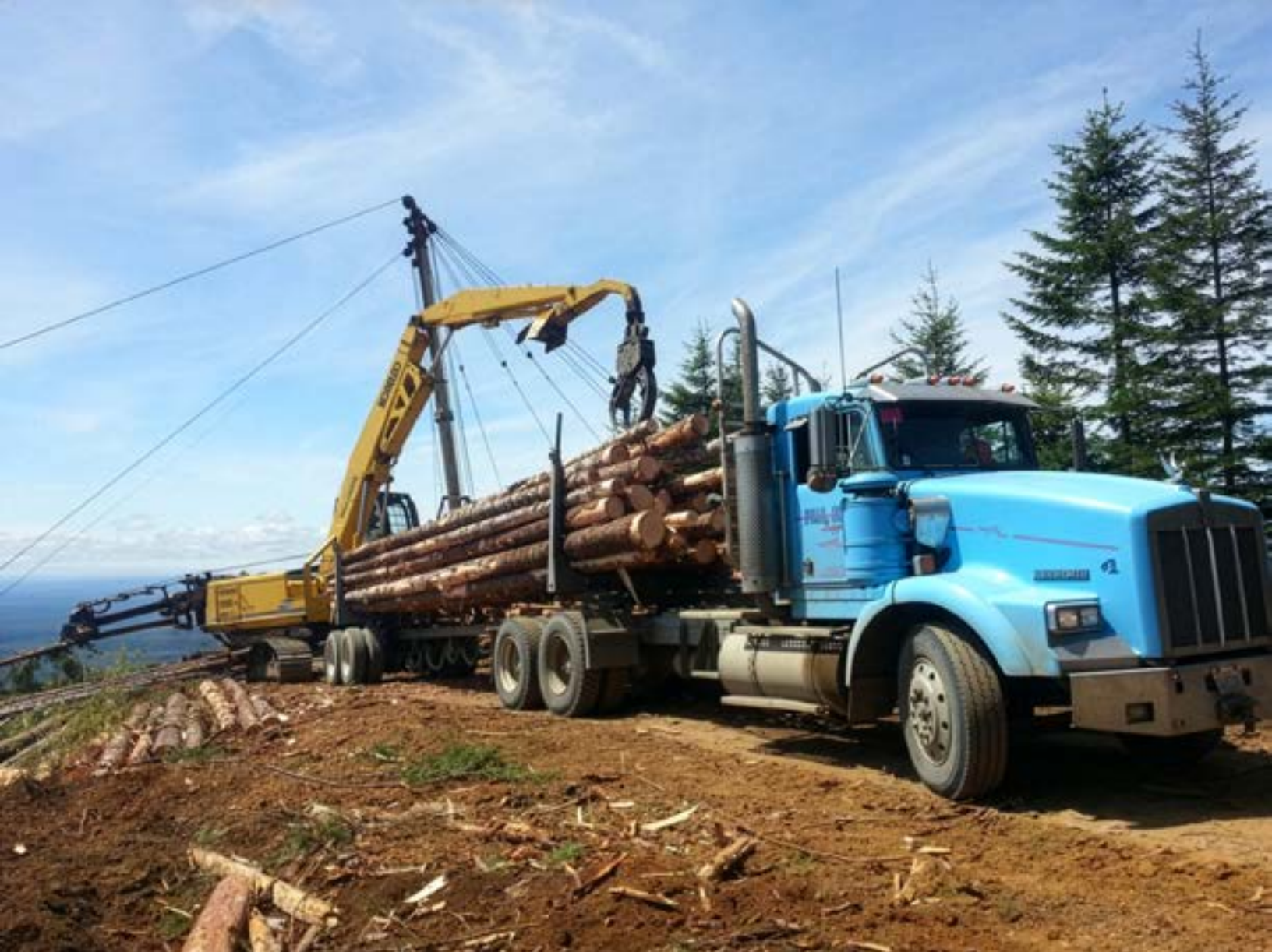
Log loader loading a truck with yarder and delimber in the background. Credit: John Gold
