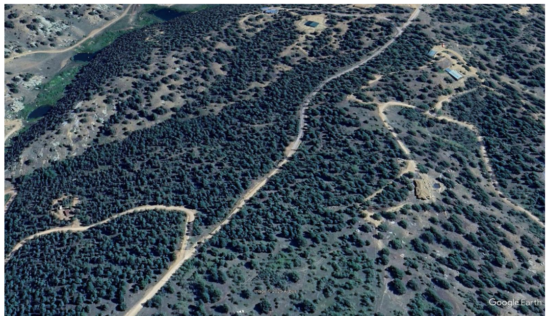
Figure 53: Examples of Non-survivable escape routes – heavy fuels on either side of the roads
